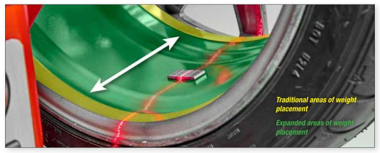
SmartWeight<sup>®</sup> Elite vision system increases balancer accuracy and single weight solutions.
