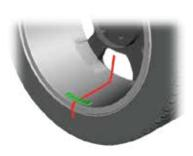
TruWeight<sup>®</sup> provides live navigation through selection and placement of wheel weights
