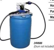
**Pump Technical Husky 515 AODD Specifications Maximum Flow Rate** 15 gpm **Maximum Fluid Pressure** 50 psi **Air Operating Range** 30-50 psi Air Inlet 1/4" NPT(f) **Pump Inlet** 1/2" BSPP(f) and 3/4" BSPP(f) Hose Inlet 3/4" BSPP(f) 1/2" BSPP(f) and 3/4" BSPP(f) **Pump Outlet Maximum Air Consumption** 28 scfm
