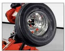
✓ Bead loosening and demounting can be as easy as rolling the tire off of the rim in a single step
