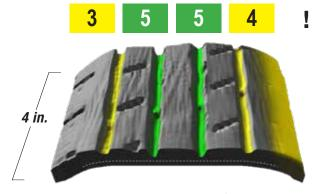
Accurate tread depth calculated for each groove.
