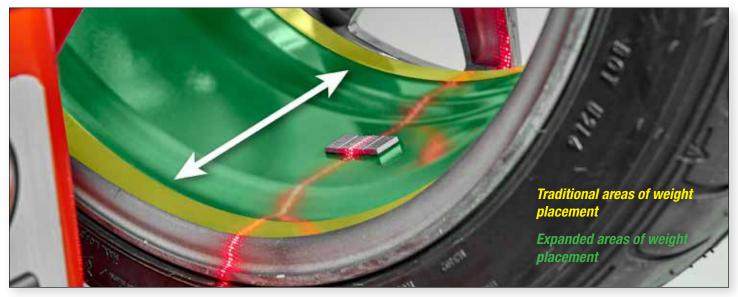
Road Force Elite vision system increases balancer accuracy and single weight solutions.
