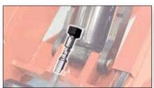
Instantaneous shutdown in event of hydraulic failure
